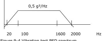
Figure 9-4 Vibration test PSD spectrum
