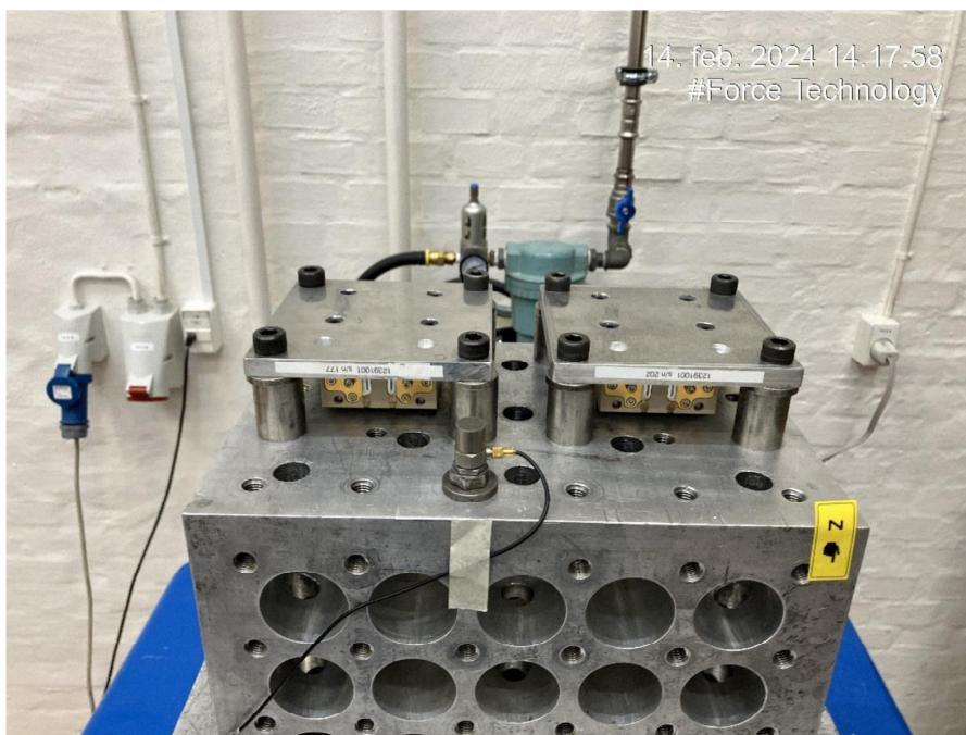
Photo 28 Test setup on shock machine for shocks in negative Z-axis. Another run with the other two test objects performed to complete all the shocks.
