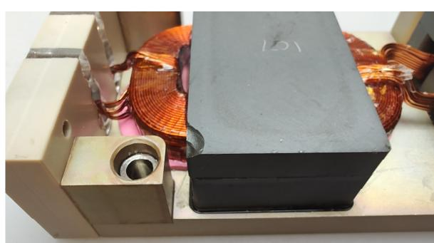
Due to the size of the unit it was not possible to microsection the transformer. All parts were examined externally and then 1 unit deconstructed.
