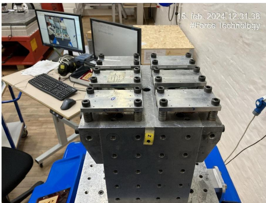
*Photo 25      Test setup on shock machine for shocks in negative Z-axis. Several runs performed to complete all the shocks.*
